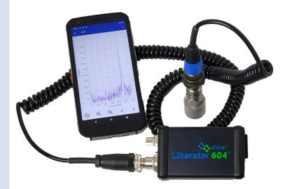
needs to be used to collect vibration data. Upon route completion, the vibration readings are uploaded into MAINTelligence $^{\text{\tiny M}}$  for alarming and analysis.
